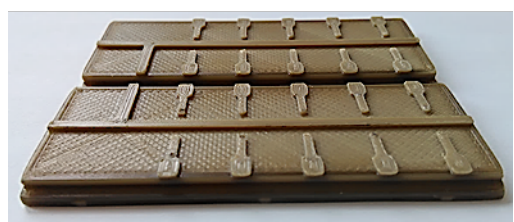
Figure 5. 3D printed mould inserts made of PEEK.
