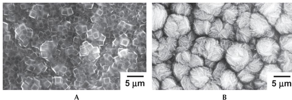
Figure 4. SEM micrographs of diamond and GF-like carbon synthesized by changing the substrate temperature and reactant ratio of  $\text{O}_2/\text{C}_2\text{H}_2$ . (A): diamond at 1123 K and 0.90, (B): GF-like carbon at 1423 K and 0.80.
