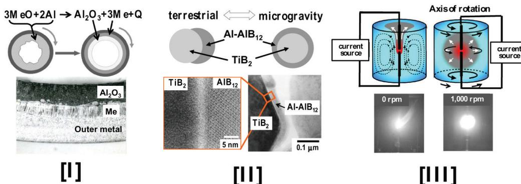
Figure 1. SHS related technologies applied under various inertia force conditions. [I]: Centrifugal-thermite process, [II]: Microgravitational SHS, [III]: Swirling chamber method.
