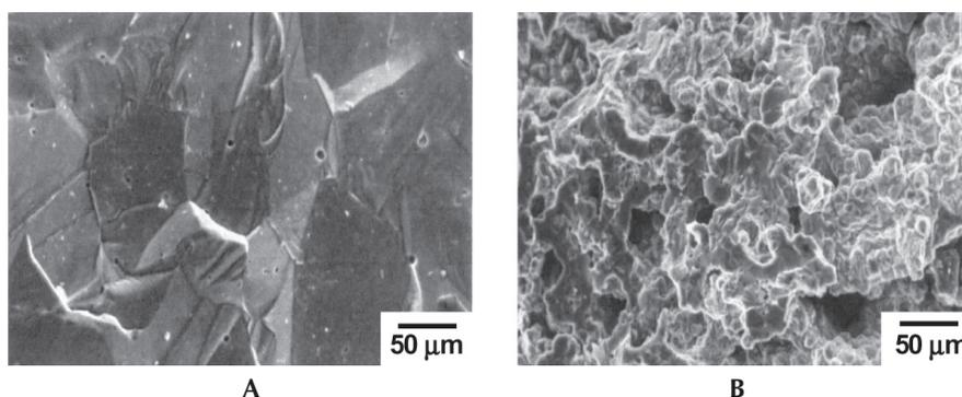
Figure 3. SEM micrographs of product fracture surfaces obtained by TiN SHS with liquid nitrogen. (A): under closed condition, (B): under atmospheric condition.
