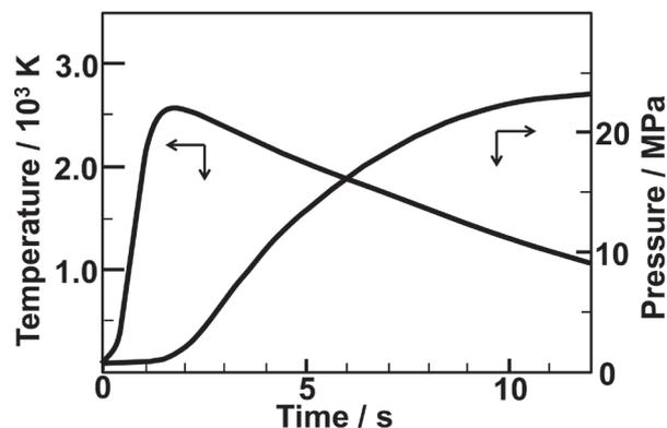
Figure 2. Typical experimental results of sample temperature and pressure inside the vessel during the TiN SHS experiment in the closed vessel filled with liquid nitrogen.
