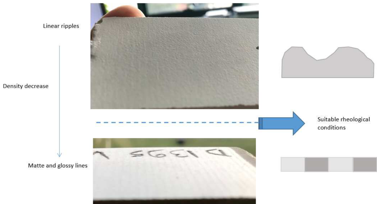
Figure 7. Defects observable on the surface of a 277B tile sample: linear ripples at high densities an alternative glossy/matte pattern at low densities.
